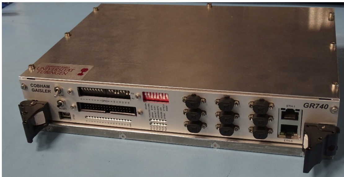
Figure 3.11: Prototype of the LAD’ s Instrument Control Unit (ICU), developed by the University of Tübingen, based on a LEON4 – GR740 Evaluation Board.
