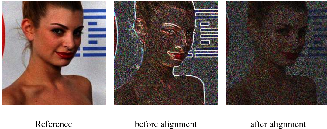
Figure 6.6: Alignment error between the reference and the last burst image scaled 5 times. Note, how after alignment, differences in the silhouette are no longer present.
