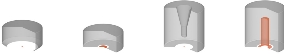
Figure 3.3.: Contact geometries of different detector types. The p^+ contact is shown in orange, while the n^+ contact is grey, separated by a white groove or passivated surface, depending on the detector type. From left to right: PPC, BEGe, ICPC, Coax. (From [36])
