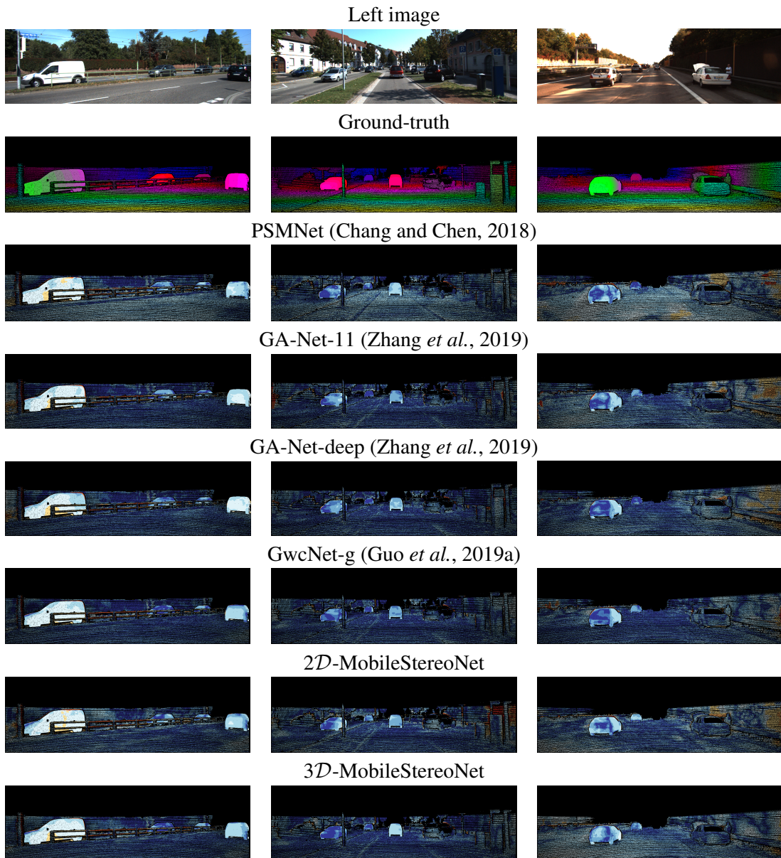
Figure 4.9: Qualitative performance on KITTI 2015 validation set: From top to bottom, the left image, the ground-truth disparity map and the estimated disparity maps by PSMNet (Chang and Chen, 2018), GA-Net-11 (Zhang et al. , 2019), GA-Net-deep (Zhang et al. , 2019), GwcNet-g (Guo et al. , 2019a), 2D-MobileStereoNet and 3D-MobileStereoNet are illustrated. For a fair comparison, we trained all the models with a 160 training and 40 test images of the KITTI 2015 training set. Warmer colors in error maps denote higher errors.
