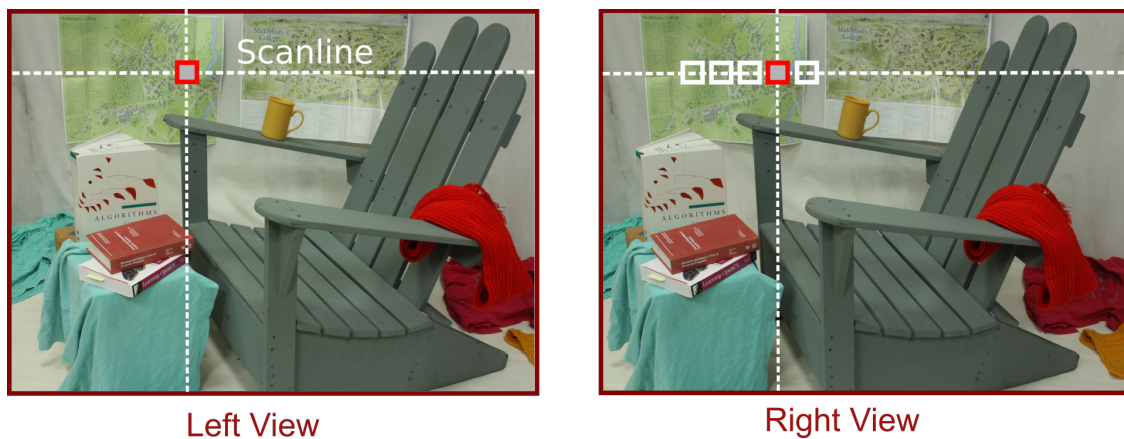
Figure 2.8: A visual representation of the feature matching process. Features from the left image are matched along the epipolar line in the right image to identify the corresponding patch. Images from Middlebury dataset (Scharstein et al. , 2014) are used to draw this figure.
