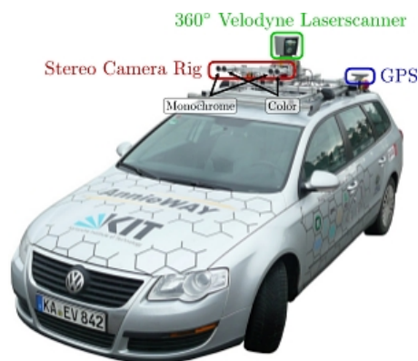
Figure 2.13: Recording platform used for capturing the KITTI Benchmark Suite dataset (Geiger et al. , 2012). The vehicle is equipped with diverse a set of sensors.
