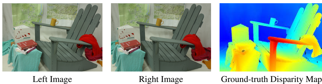
Figure 2.16: An example of a stereo pair and its corresponding ground-truth label from the Middlebury dataset (Scharstein et al. , 2014).
