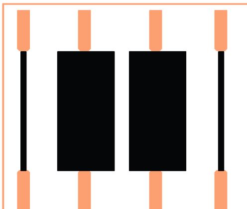
(a) Schematic drawing of the silicon double module. The wafer detectors are also silicon phonon detectors [Credit: CRESST Collaboration].
