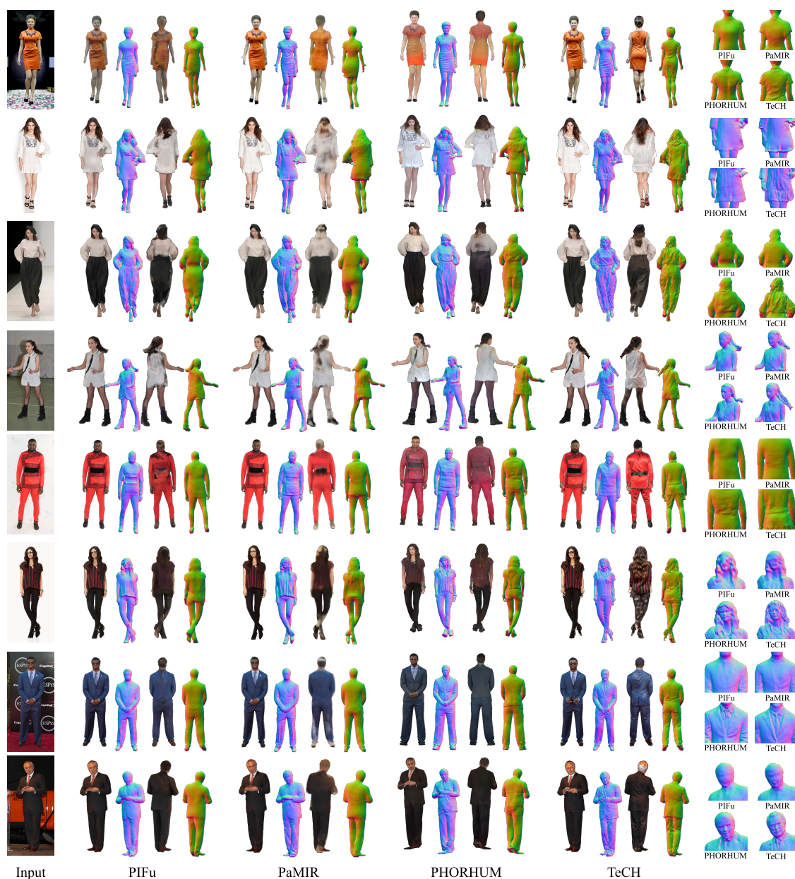
Figure C.3: Qualitative comparison on SHHQ images. TeCH generalizes well on in-the-wild images with diverse clothing styles and textures. It successfully recovers the overall structure of the clothed body with text guidance, and generates realistic full-body texture which is consistent with the colored pattern and the material of the clothes. Q Zoom in to see the geometric details.
