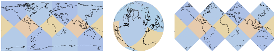
Figure 4.10: Coastlines of our planet in the equirectangular Mercator projection (left), on the sphere (center), and in the distortion-reducing HEALPix projection (right). On a distortion-free representation, Greenland should fit roughly seven times into South America, which applies to the HEALPix, but not to the equirectangular representation. Color codes indicate how HEALPix divides the sphere into twelve faces: Four each on the northern and southern hemisphere (blue), and another four around the equator (orange).
