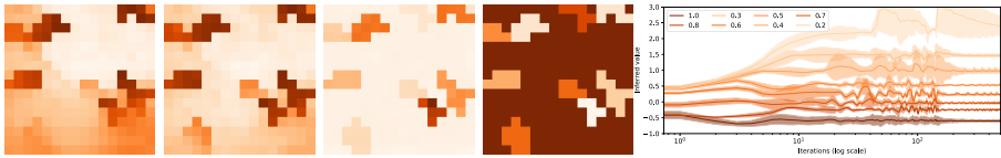
Figure 4.3: Inference of water depth when simulating the SWE. From left to right: Iteration 1, 2, and 500 of the inference procedure with inverted value range in \mathbf{c} compared to the ground truth shown in the fourth panel. In the rightmost panel, the inference process of the water depth values is visualized. Figure modified from Karlbauer et al. (2021).
